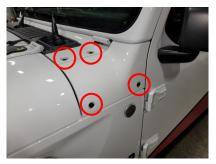
**2. Install Foam to Bracket:** Remove the backing from the protective foam and place it as shown below. This foam will help protect the paint of the Jeep under the brackets.
