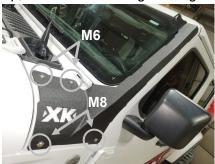
**4. Mount 50" Light Bar Spacer (if applicable):** Install the spacers to the A-pillar brackets using the provided hardware. These allow for perfect fitment for 50" light bars.
