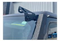
5. Install Light Bar: Use the bolts provided with the light bar to mount it to the Jeep. Be sure to check the clearance of windshield wipers to the light bar before finishing the installation. Use the slotted adjustments in the a-pillar brackets to try different light bar positions to best suit for visibility and wind noise.
