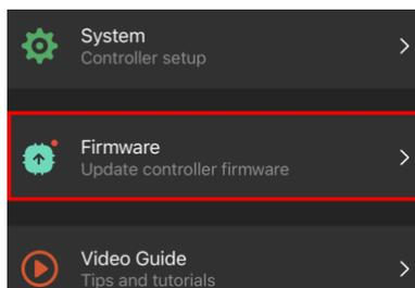
**Firmware-** Firmware on XKcommand can be updated via Bluetooth. Red dot will appear when new firmware is available. When updating, ensure XKcommand is powered ON until update is complete.
