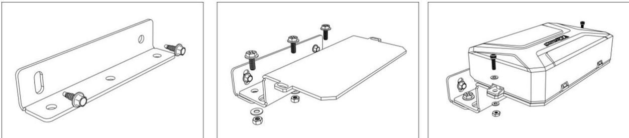
After the hub is secured, remove the hub cover by pressing the tab shown below in **GREEN** and rotating it towards the rear.
