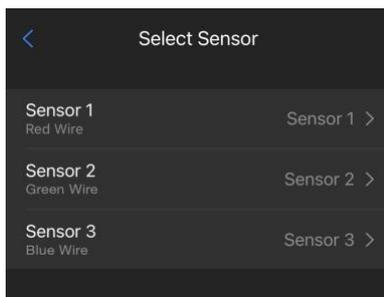
From the **Customize** menu, select **Sensor Wire**. Choose which sensor wire to customize from the screen above. Wire color can be seen below each sensor wire.
