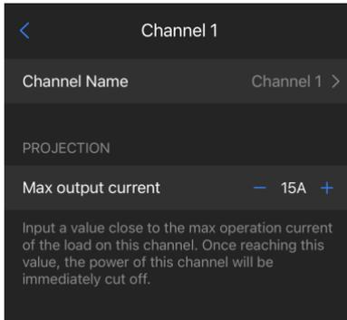
Under the **Output Channel** menu, set the current limit for each channel.
