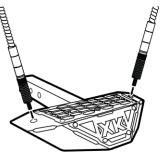
3. Install Hitch to Receiver: Connect all wiring and run wires into the tube of the hitch step. Insert the hitch step into the hitch receiver of the vehicle with the supplied locking hitch pin. Then connect the 4-pin connector. Test the lights and both turn signals to ensure they are connected properly. \*If the turn signals are opposite of the vehicles, swap the whip connections going to the controller.
