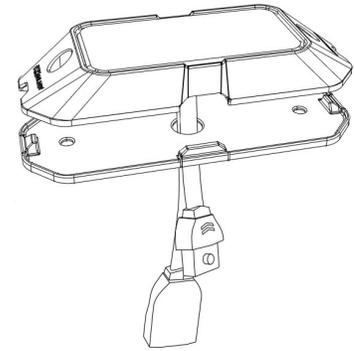
2. **Optional- Mark and drill for Through-Hole Wiring:** If utilizing the through-hole wiring method, mark and drill a 3/4" hole in the center of your desired mounting location.
