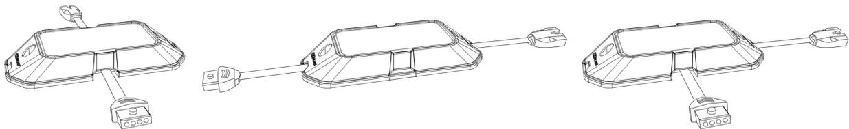
Select two of the four tabs on the rubber grommet for the wiring to feed through. These will be for the input and output wires. Choose what best fits selected pod in its desired mounting location and using a pair of scissors or a razor blade, carefully cut off the two tabs. Leave the remaining two tabs in place to prevent dirt/grime buildup under the pod.
