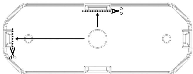
**Option B. Through Hole Wiring:** If you can access the rear of the panel you are mounting to, you can utilize the through-hole wiring method. Simply drill a 3/4" hole in your desired mounting location and feed the wiring through to the rear of the panel. This method can be seen to the right.
