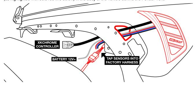
3. Tap into factory sensor wires and connect to power: The three side facing light bars are controlled with the vehicle turn and running light signal. Use the diagram below to locate the Running Light, Turn Signal Light, and Ground wires from the factory wiring harness. Use provided T-tap connectors to tap into corresponding wires. Connect the white wire to vehicle 12V+ battery power.
