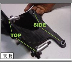
9) Carefully pu into place the ZROADZ Mounting Brackets to Jeep JL A-Pillar. Check for clearnaces and proper placement of gaskets for coverage and protection of vehicle finish. Route & hide the Roof Level LED Light Bar Power Hamess down the Vehicle's A-Pillar behind ZROADZ Mounting Bracket. Use the provided M6 x 50mm Round Head Black Screws to secure
