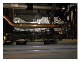
**Step 4**: The included Connector Pipe is required for the four door model only. It is to be installed between the Resonator Assembly and the Over-Axle Pipe. if you have the two door model this pipe may be discarded.
