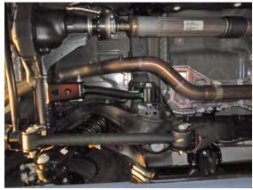
**Step 5**: Next, loosely install the Over-Axle and Extension Pipe Assemblies using the supplied 3.00" clamps. Locate welded hanger to the rubber insulator.
