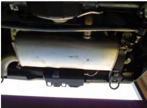
**Step 2**: With the system supported, working front to rear disengage the hangers from rubber insulators and remove the OE system. Do not discard or damage the clamp or rubber insulators as they will be used to install the new system.
