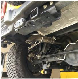
**Step 6**: Next attach the Tailpipe Assembly (either the Side Exit or Turn Down) to the Over Axle Pipe Assembly with the supplied 3.00" clamp and fit the hanger into the rubber insulator.
