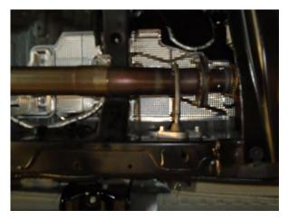
**Step 3**: Begin installation of your new MAGNAFLOW system by attaching the Resonator Assembly to the flex pipe using the supplied Fasteners. Engage the welded hanger to the rubber insulators. Keep all fasteners and clamps loose until final adjustment.
