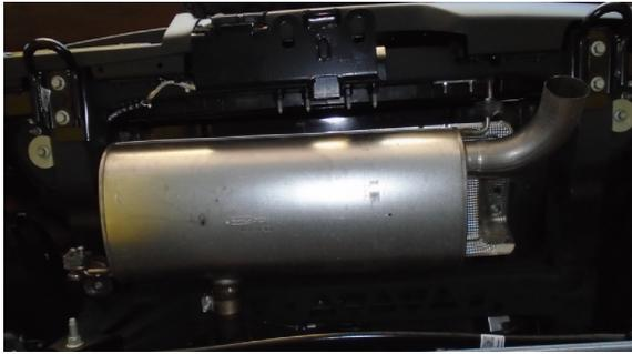
Step 1. Remove the OEM system by first loosening the factory TORCA clamp on the overaxle pipe. Next disconnect the rubber hangers and set the muffler to the side.
