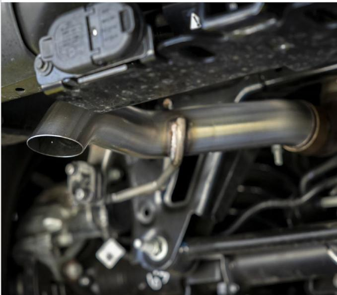
Step 2. Slide the MagnaFlow tailpipe into the factory overaxle pipe, and then slide the hanger into the rubber isolator.
