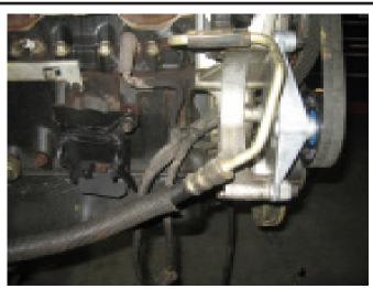
The LT1 engine can be used with the bolt in YJ mount as long as you replace the A/C pump with the Chevy P/N 10115875. This is a replacement pulley for the LT1 that removes the A/C pump. The replacement pulley is slightly smaller in diameter and will require a new belt.
