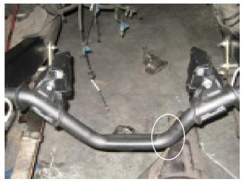
The P/N 713087 mount is designed around a stock Jeep front axle. The photo above shows the mount with a Jeep that has a custom axle installed. The interference is due to the size of the axle housing and the lift that is installed. The axle is installed under the springs, a spring over on this axle would provide ample clearance for the mount. This is just an example of a potential interference problem.
