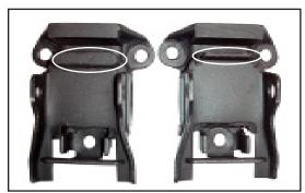
There are two style of GM mounts that we receive from our supplier. The mount on the right fits our mount correctly, the mount on the left requires a slight modification to the rubber portion circled. These mounts are listed though GM as the same part number.
