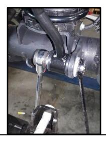
**5.** Using a silver marker, draw index lines onto the front drive shaft at flange. This will ensure proper alignment and balance of the drive shaft when reinstalled. Using a 15mm socket, remove the front drive shaft flange from differential. **NOTE:** Suspend drive shaft from vehicle using cord, wire, or bungees. **DO NOT ALLOW drive shaft to hang**, as damage to rubber butt may result.
