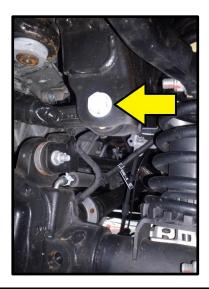
**4.** Using an 18mm socket and wrench, remove the lower bolts to sway bar links. **Do not discard OE hardware.** It will be reused. Repeat for the other side.
