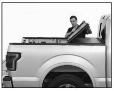
C. Always ensure all latches and hooks fully engage side rails. Close tailgate.
