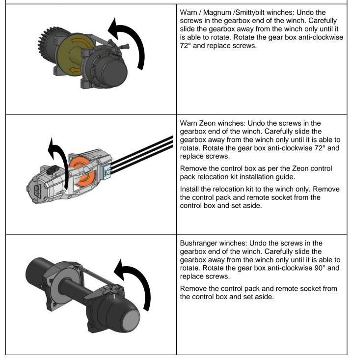
*If fitting a Bushranger or Zeon winch continue from here. If not continue to install the winch as per fitting instructions 3787989 supplied with kit 3540050. The following pictures show the Zeon plug and plug cover. The same steps apply for fitment of Bushranger winches.*
