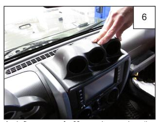
Apply firm pressure for 30 seconds on each section of the part to ensure proper adhesion.
