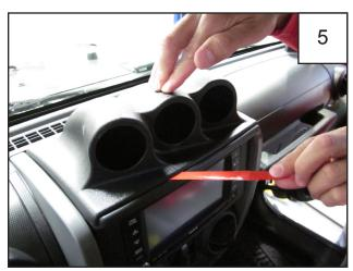
Pull liner of lower 1/2" tape strip. Press down on entire length of the part again applying firm pressure to the taped areas. *NOTE: The tape reaches maximum adhesive bond after 24 hours of contact.*
