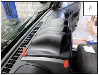
It is recommended that you align the part on the dash an equal distance between the front and the back edges. NOTE: Alignment between front and back edges is adjustable based on customer discretion.
