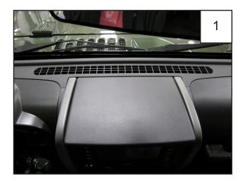
Clean all dirt and debris from dash. Dry fit the pod on the dash, and determine how you will run your gauge wiring. This pod can be used with or without gauge brackets. If no brackets are used, you can leave the gauges out until the pod is mounted, however wiring must already be in place and easily reachable. If you chose to use gauge brackets must already be mounted and wired before mounting the pod.
