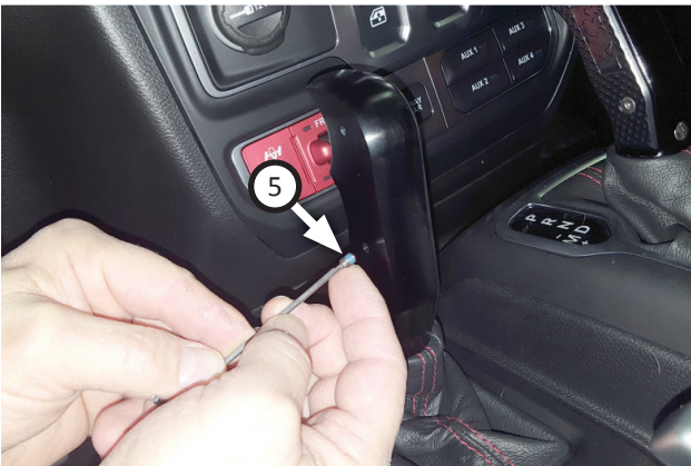
26. Apply loktite to set screw (5) then install into transfer case handle as shown.
