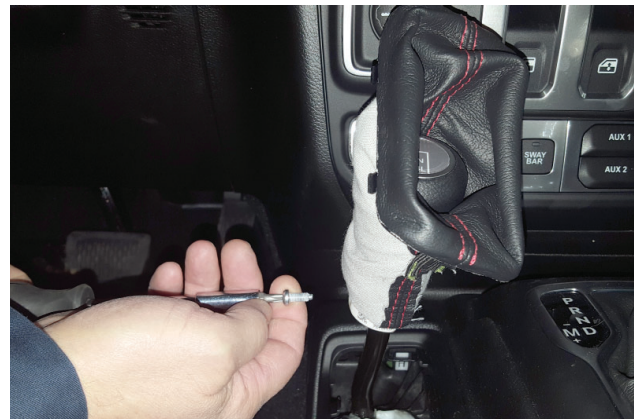
17. Remove screw from transfer case shifter knob as shown.
