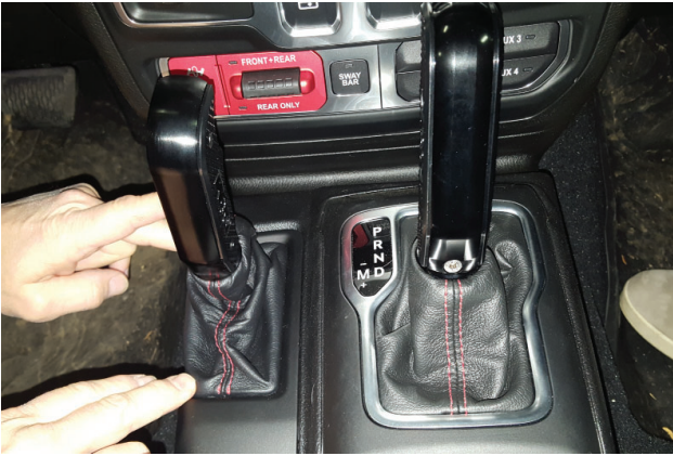
24. Clip boot cover into console cover as shown.
