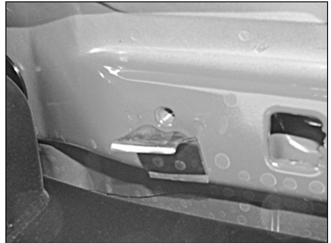
(Fig 2) 8mm threaded hole in floor frame channel (passenger side-front pictured for example)
