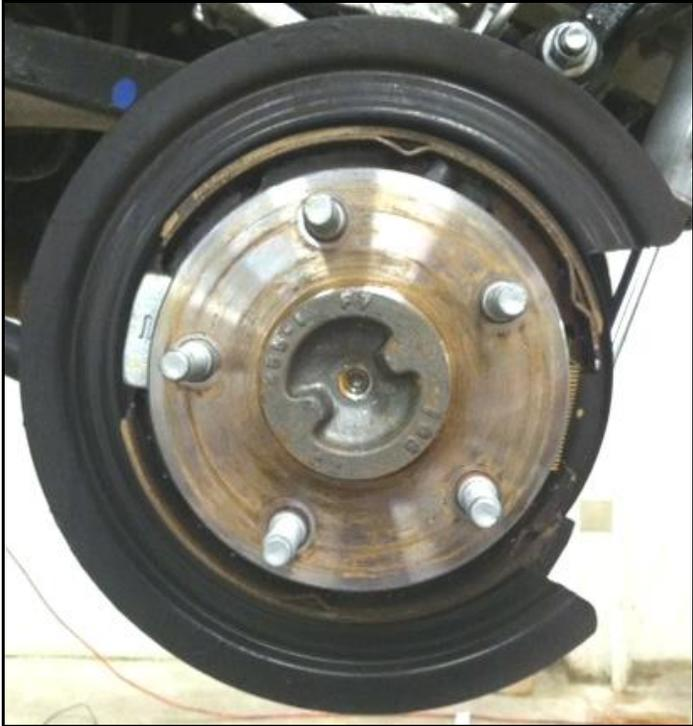
**Figure 2:** Front view of dust shield after trimming
