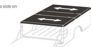
Affix the center panel to the truck by placing a **cap clamp** at each of the four interior corners of the underside of the center panel and tightening them with a 9/16" socket (or wrench for Titans).
