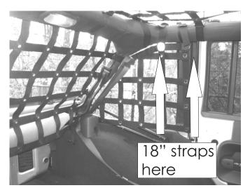
To install the bottom strap you need to pull back the carpeting from the rear quarter panel. Pass the webbing trough the bracket as shown and connect into ladderloc on side net.
