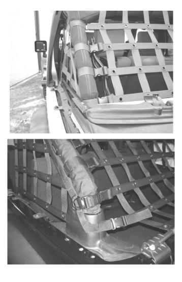
Slide each half of the tailgate bar in the last row as shown in the photo. This bar will connect at the center of the net and then the whole bar is clipped into soft-top tailgate clips. (Clips can be purchased form us or your local dealer.) This last row is optional and can be cut off if not needed.
