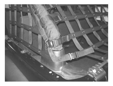
Any excess straps that hang out can be tucked in under it's self. Adjust and tighten straps as needed to even out the net so it is positioned properly. Your net comes with a 3 year warranty against manufacturing defects. Cuts, abrasions, sun faded items are not covered under the warranty.
