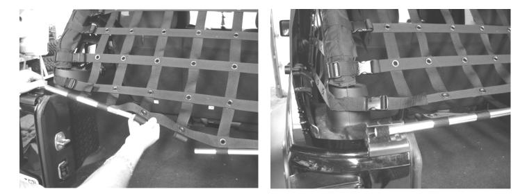
The strap at the very top of the rear piece wraps around the top of the vertical roll bar comes toward the outside wraps back around and connects into the ladderloc clip. See photo
