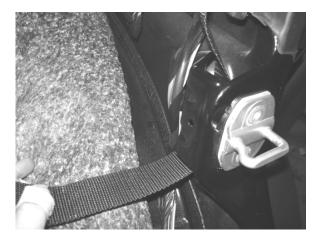
Rear corner of the side gets clipped into the buckle off the back piece.
