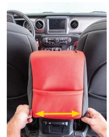
Place the console lid cover over the console starting from the top keeping the Diver Down tag to the bottom left. Using both hands, align the keyhole from the top and slowly work the console lid cover to the bottom. (Fig 3) **Note:** the bottom of the console will have a space to fit the rest of the cover when the console is kept in the raised position. Secure the console lid cover on the bottom of the lid using both hands. (Fig 4)
