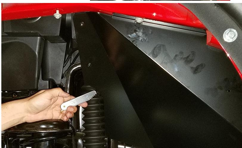
4) The arm will go behind the bulk head that the liner is up against. This picture is illustrating the approximate location the arm need to be resting at.
