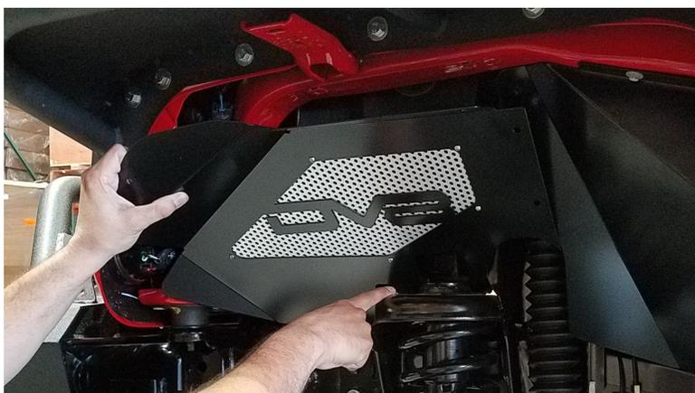
7) Next step is aligning the two halves. To do so push back on the two halves until the holes line up to screw in the two stainless short screws. Once those two screws are in and tight, you can fully secure the front section.
