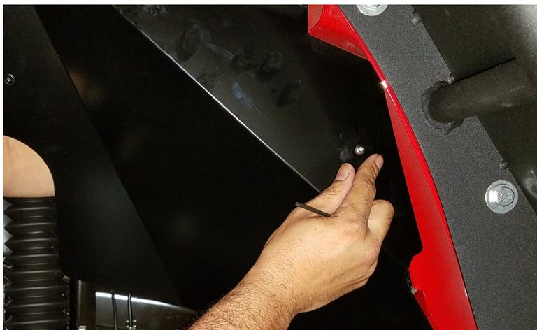
6) Now you can install the front half. (part that has the DV8 cut out of it) Place the liner in bottom first just behind the spring perch. Secure it loosely with the factory bolts. Up top two bolts and front fender spot. (Wire the second light up through the engine bay at this time. )
