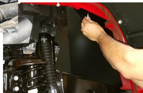
3) Next take the arm that comes with the parts kit and place it behind the panel. Needs to be in the orientation in the picture. Threaded part of the nutsert facing the motor. You should have a right and left arm.
