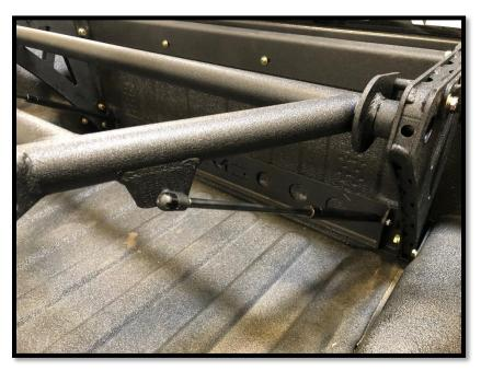
9. Lastly install the tire mount as shown. Once secured, you can install you wheel and tire combination.
