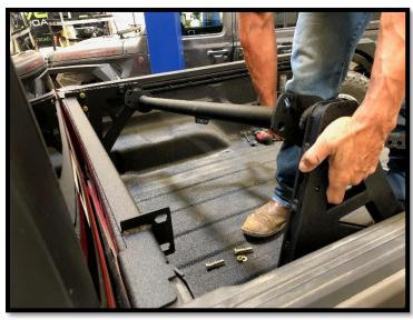
7. Tighten all hardware at this point. Main carrier tube should easily move up and down. Next, secure bolt pull locks into place using provided hardware. Make sure to put pull lock into one of two holes on main center tube before securing. NOTE: These may need to be tapped into placed initially. This is normal.
