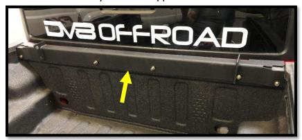
4. Install the lower support. The lower support has two holes on each side. The front hole with the factory threaded hole in the bed is required, the second hole that is through bolted is optional for tires larger than 40".
