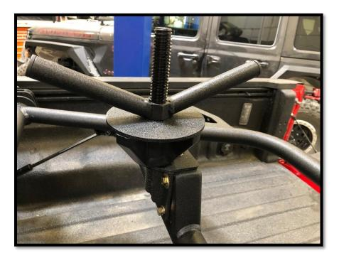
10. Install the tire faced up on the post. Then place the rubber cone, round plate, and finally the screw handle.
