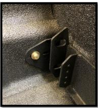
5. Once both support bars are installed, place the passenger side mount into place as show and loosely install hardware. This needs to be able to move to get the main carrier and driver side mount installed.
