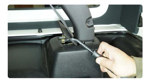
STEP 17 Use the trim tool to separate the panels at there parting line.
