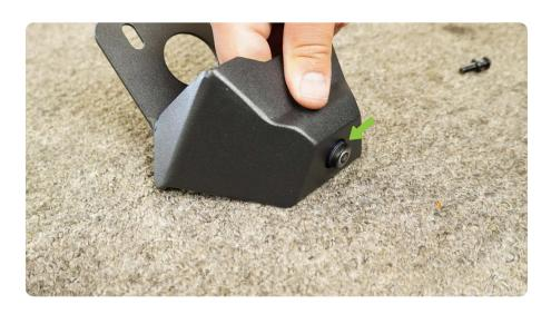
STEP 38 | Using a #4 allen and 10mm wrench with the provided M6 allen head hardware, secure the rear camera in the camera housing.
