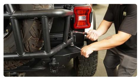
STEP 52 | With the mounting bracket aligned, mark the upper, middle and the bottom holes that will need to be drill out.
