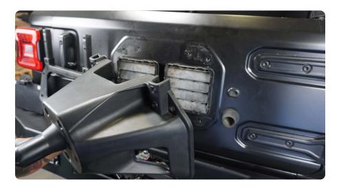
STEP 6 | Open the tailgate and use a T40 torx tool to remove the torx head bolt that secures the tailgate check cable.
