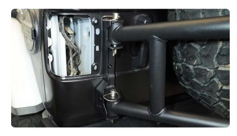
STEP 57 | Carefully install the rear taillight in the reverse order it was removed.
