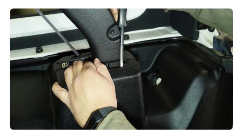
STEP 18 | Open the rear storage compartment and remove the tire jack/ tool compartment cover.
