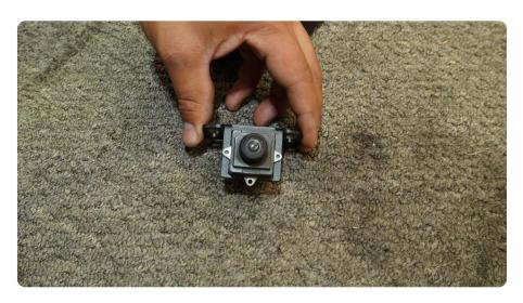
STEP 37 | Install the rear camera mount into the provided rear camera housing.
