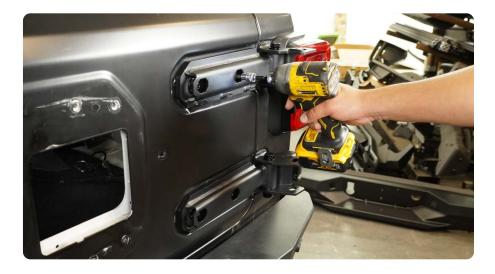
STEP 34 | With hinges installed and tailgate secured we can now assemble the tire carrier.
