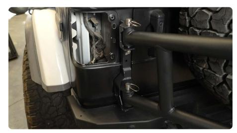
STEP 49 | Ensure bolt upper and lower hinge bolts are loose enough to be adjusted.
