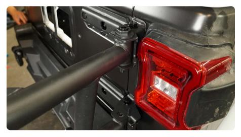
STEP 43 | Loosely secure the bottom of the cage to the lower hinge using the provided M14x35 hex bolt.
