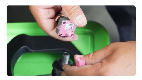
STEP 12 | If you vehicle is equipped with the newer camera style shown, depress the camera from the camera mount, unplug the camera harness and set everything off to the side.
