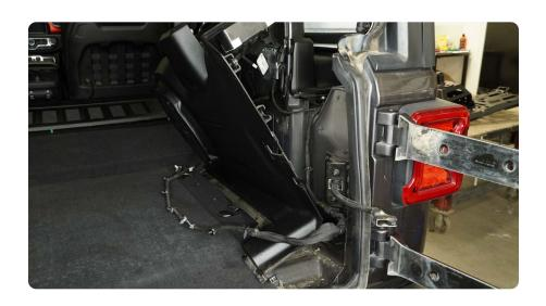
STEP 24 | Remove the factory hing cover stickers to gain access to the (6) hinge bolts.
