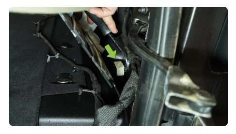
$\begin{array}{c|c} \text{STEP 20} & \text{I} & \text{Use the trim tool to pry the} \\ \text{panels last clip.} \end{array}$
