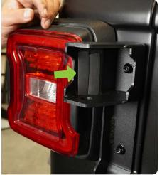
STEP 60 | Place the provided foam strip in the center of the tailgate vent cut outs.
