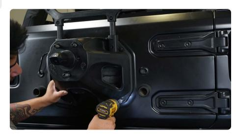
STEP 2 | Use a T25 torx bit to remove the hardware securing the third brake light to the tire carrier.
