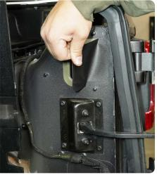
STEP 25 | Use a 13mm socket to remove the (6) factory hinge bolts. Set the factory hinges off to the side, they will not be reused.
