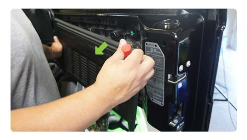
STEP 8 | Unclip all three plugs to the camera, third brake light and tailgate door handle.
