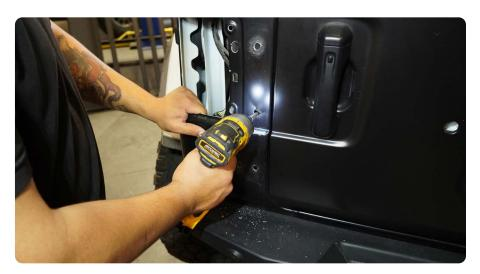
STEP 54 | Place the provided support bracket into the body panel through the tail light cut out with the flat side of the nutserts faced towards the rear of the vehicle.
