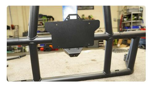
$\begin{array}{c|c} \text{STEP 41} & \text{with assistance, slide the} \\ \text{cage bushings into the hinges, starting} \\ \text{with the bottom then the top.} \end{array}$
