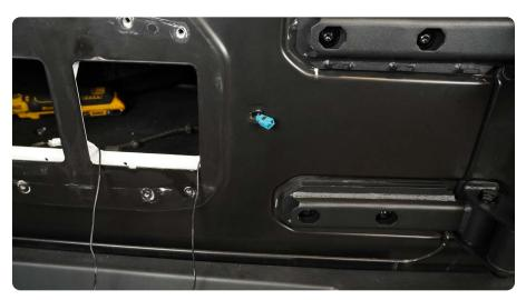
STEP 45 | Feed the extended harness through the tire carrier cage tube.
