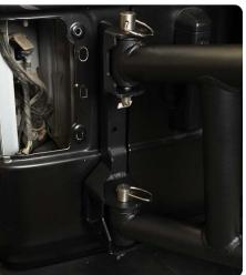
STEP 50 | The driver side mounting bracket should be 1/8 inch away from the edge of the body panel.
