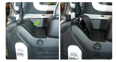
STEP 22 | Using a 10mm socket, loosen the plastic tail light bolt.
