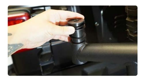
STEP 59 | Place the provided rubber stop strips into the upper mounting slot on the driver side bracket.
