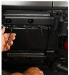
$\begin{array}{c|c} \text{STEP 47} & \text{Mount your spare tire onto} \\ \text{the cage tire carrier.} \end{array}$
