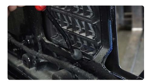
STEP 10 | Using a Dremel or cutting tool of choice, remove the three sided border from the fin vents.
