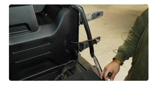
STEP 15 | Use a T20 torx tool to remove the factory torx head bolt that secures the rear trim panel/sub-woofer.
