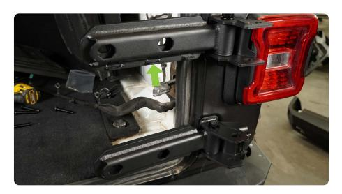
STEP 32 | Mount the tailgate back onto the vehicle aligning the vehicles body lines.
