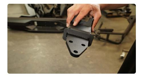
STEP 27 | Before mounting the DV8 hinges, place a small mount of blue thread locker to each of the (6) factory hinge bolts.
