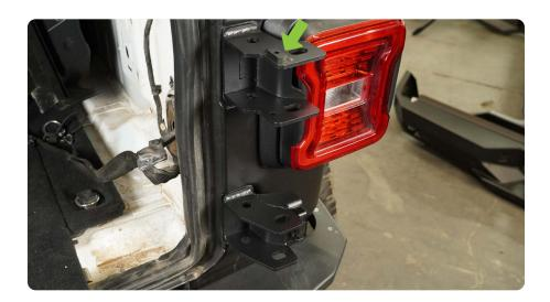
STEP 30 | Place the provided foam pieces on to the back of the hinge arm as shown.
