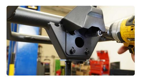
STEP 40 | (Optional) If you wish to relocate your license plate to the tire carrier cage, use the provided license plate bracket to do so.
