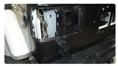
**STEP 56** Close the carrier to check alignment. The carrier should have some pre-load.
