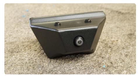
STEP 39 Using a 13mm socket or wrench, mount the rear camera housing to the bottom of the tire carrier cage center plate. Using (4) of the provided M8x25 hex bolts.
