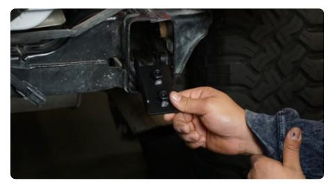
STEP 12  $\mid$  Lift the bumper to the vehicle and loosely secure using the factory hardware and a 21mm or 18mm socket.
