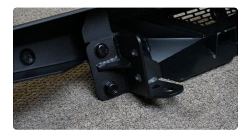
STEP 11  $\mid$  Slide the nut plate into the passenger frame rail lining it up with the mounting holes on the bottom.
