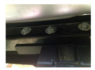
11) Tighten the 4 side bolts that are loosely inserted into the nut plates with a ratchet. Torque to 60 ft/lbs
