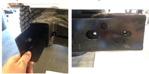
7) Next insert the 4 large 3"x 12mm through bolts through the frame rail with the threads facing the rear of the Jeep, make sure to put the washers onto the bolts as well. NOTE: You'll have to put the head of the bolt above the exhaust canister to get it into the hole.
