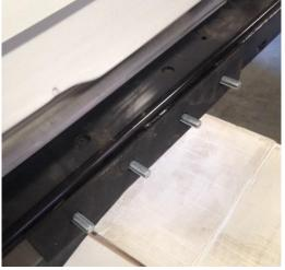
9) Have a friend or two lift the bumper with you and place the holes in the middle of the bumper on to the bolts sticking out of the rear of the frame. Install the nylon nuts on the 4 through bolts sticking out of the rear to hold the bumper to the frame. Next, install the shorter bolts through the sides of the bumper and into the nut plates you previously in-
