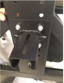
16) Place the final piece of the tire carrier into the slot shown below and use the two bolts provided to loosely attachit.
