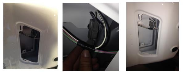
4) Next, remove the rubber plug and wire from the tailgate that is connected to your rear brake light. The plug should pull through if you disconnected the wires correctly. If it is not
