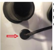
coming out easily, help the rubber fitting from the inside of the tailgate by pushing from the rear and pulling at an angle downward at the same time. 5) Remove the factory spare tire carrier by removing the 8 bolts (13mm) attached to the tailgate.
