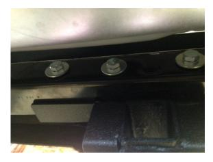
11) Tighten the 4 side bolts that are loosely inserted into the nut plates with a ratchet. Torque to 60 ft/lbs
