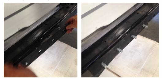
9) Have a friend or two lift the bumper with you and place the holes in the middle of the bumper on to the bolts sticking out of the rear of the frame. Install the nylon nuts on the 4 through bolts sticking out of the rear to hold the bumper to the frame. Next, install the shorter bolts through the sides of the bumper and into the nut plates you previously in-
