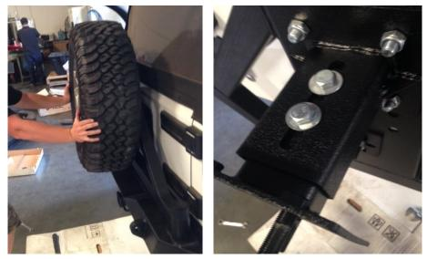
21) Now that everything is tight put your spare tire back onto the studs and secure it using the factory lug nuts. And you're finished!
