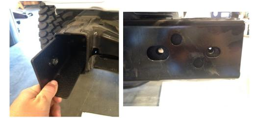
7) Next insert the 4 large 3"x 12mm through bolts through the frame rail with the threads facing the rear of the Jeep, make sure to put the washers onto the bolts as well. NOTE: You'll have to put the head of the bolt above the exhaust canister to get it into the hole.
