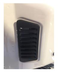
3) Once the vent is off, locate the small wiring harness just inside the vent and unclip it. This is the wire to the factory third brake light.
