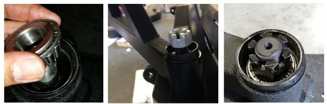
15) Next step is packing the bearings with grease. Once bearing is packed, turn the carrier upside down and place the large bearing in the bottom of the carrier, small side first. Next, install the seal over the bearing by tapping the seal in with piece of wood across it and a rubber mallet. NOTE: It's ok if peels away a little rubber off of the seal when tapping it in.
