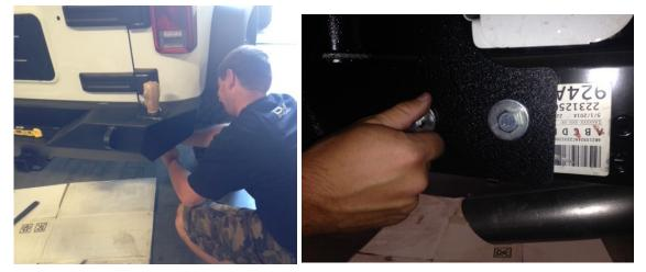
12) Ensure that the bumper is level. If it is not level repeat steps 12-15 making adjustments to level the bumper. NOTE: If the bumper is not level have a friend hold it level and tighten the side bolts first and then tighten the rear cross-member bolts. The bumper should be mounted as level as possible.
