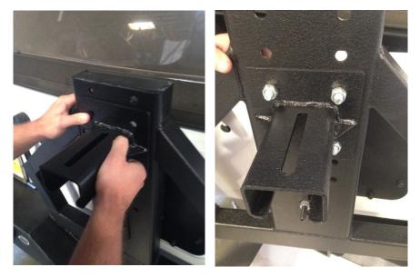
19) Place the final piece of the tire carrier into the slot shown below and use the two bolts provided to loosely attach it.
