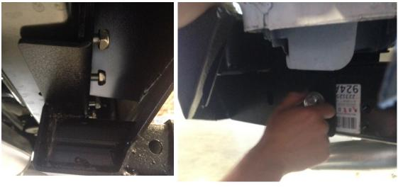
10) Next tighten the four center bolts in the rear cross-member first to allow the bumper to properly align itself. Torque to 60 ft/lbs.
