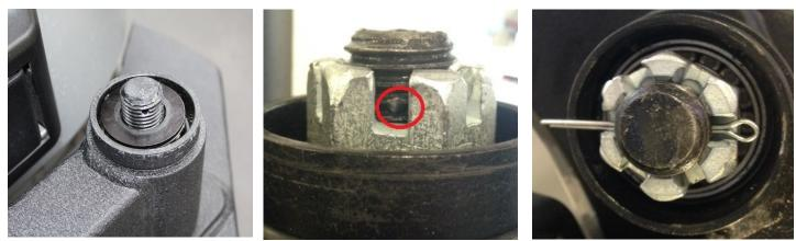
17)Bend the end of cotter pin to secure. Set the cap onto the whole assemble with the holes lined up that are highlighted below and then insert the small tapered head screw and tighten.
