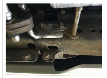
**Step 2.** Begin installing your new Axle Back system by mounting the supplied Hanger Bracket OVER the OEM hanger and fasten using the supplied M8 nuts.
