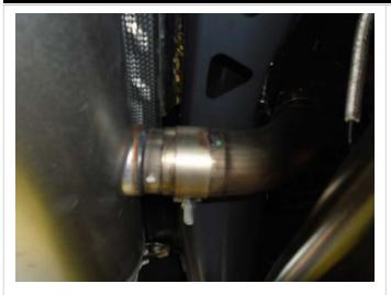
**Step 1.** Remove the OEM muffler assembly by first loosening the clamp attaching the muffler inlet to the midpipe. Disengage the two welded hangers from the rubber insulators. The muffler assembly may now be removed.
