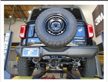
**Step 5.** Once a final position has been chosen for the new exhaust system, evenly tighten the OEM clamp using the manufacturers torque specifications. Inspect all fasteners after 25-50 miles of operation and re-tighten if necessary.
