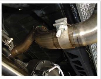
**Step 3.** Next install the OE clamp onto the Muffler Assembly insert the inlet to the OEM mid pipe outlet. Keep the clamp loose until final installation is complete.
