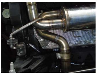
**Step 4.** Finish by engaging both welded hangers to the rubber insulators.
