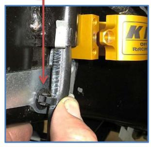
7. Now use the bent threaded nut plate included in the kit to secure the reservoir bracket on the other end. Place the nut plate in the large hole in the frame and line up with the hole in the reservoir bracket. Use the 1/4 X 1" bolts (CB4502 with washer CW1501) to thread into the nut plate.
