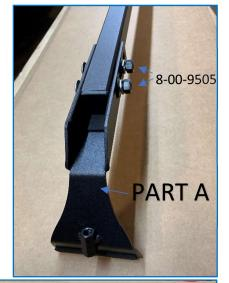
3) Now place loosely assembled crossbars on top of Vehicle so brackets sit in rain gutter channel. Center crossbar to vehicle width. Position Crossbars forward or back to your desired location from 24" to max 36" (27"-30" being the ideal spacing). On the JLU the bars fit approximately 12 inches in from the front and from the back, allowing for a 3<sup>rd</sup> bar in the middle for additional weight distribution (extra bar not included - available separately: (1) part 8-00-9651-BK with (1) 8-
