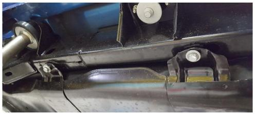
**3.** Put the Fab Fours Skid Plate in place and loosely attach it using the 4 bolts that were just removed. Bolts should be threaded approximately <sup>3</sup>/<sub>4</sub> of the way.
