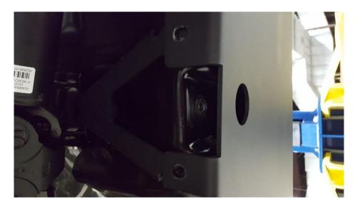
**5.** Remove the rear inner bolt on the gas tank using an 18mm socket and loosely attach the bracket by replacing the bolt. Attach this bracket to the skid plate.
