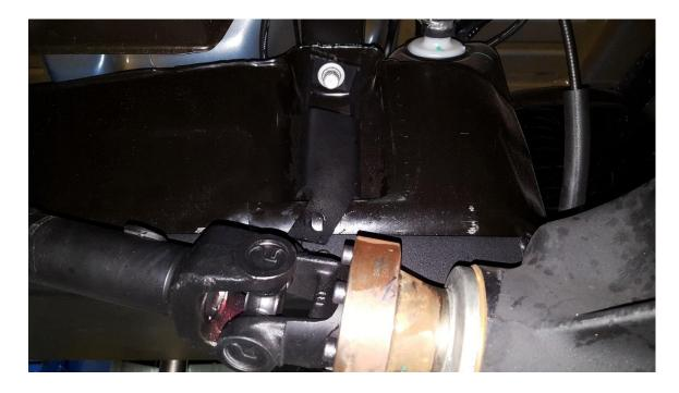
**6.** Remove the rear outer bolt using an 18mm socket and attach the bracket by loosely replacing the bolt. Attach this bracket to the skid plate with the provided 3/8" hardware.
