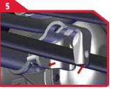
Pry apart the bracket and remove from tie rod.
