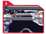
Center stabilizer body and shaft. Verify clearance and fitment between trackbar, drag link and differential
