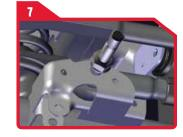
Install the provided stud in place of the track bar bolt. (Use the factory flag nut.) Torque to 220 ft. lbs.
