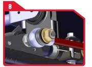
Install the Nexus EF Stabilizer evelet onto the stud using the provided nut. Torque to 90 ft. lbs.
