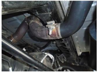
**Step 2.** Begin installing your new Axle Back system by first inserting the Muffler Assembly inlet to the OEM mid pipe outlet. Keep the OEM clamp loose until final installation is complete.
