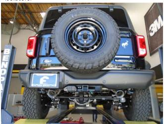
**Step 4.** Once a final position has been chosen for the new exhaust system, evenly tighten the OEM clamp using the manufacturers torque specifications . Inspect all fasteners after 25-50 miles of operation and re-tighten if necessary.
