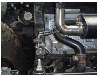
**Step 3.** Engage both welded hangers to the rubber isolators.
