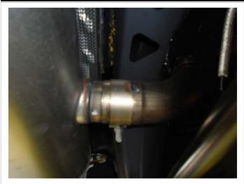
**Step 1.** Remove the OEM muffler assembly by first loosening the clamp attaching the muffler inlet to the midpipe. Disengage the two welded hangers from the rubber isolators. The muffler assembly may now be removed.
