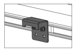
\*Line the bracket up with the tri-fold cover clamp location once they are lined up. Secure bracket to the vehicle bed rail.
