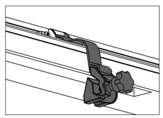
Place the assembled cover on the front end of truck bed. When the front clamps are secured, install the safety strap (see the photos). Tighten the knob of the safety straps.
