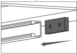
\*Attach the clamp bracket to the plate with the included Allen head bolts.
