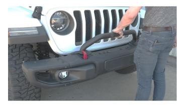
Once you have your bull-bar set in place, screw in the bolts with a T45 torx bit. Make sure your bull bar is centered with your bumper before fully tightening the bolts into place.
