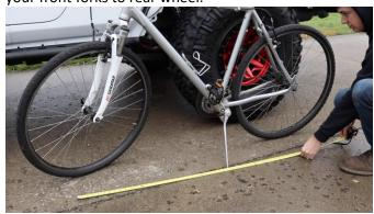
Decide which side of your rack you wish to install your bike and lay out the measurement onto the rails.
