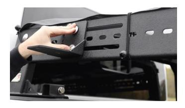
Install your wheel chock bracket with the remaining hardware at your second measurement.
