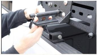
Install the mount by lining up the carriage bolt holes onto your rails, and secure it with the included carriage bolts, carriage washers, lock washers, and hex nuts (in that order) with a 19mm socket.
