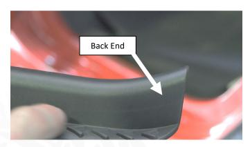
Pull away the adhesive backings located on the bottom and back end of your entry guards.
