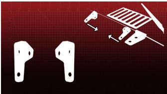
Begin screwing in the included studs into each bracket until it is flush on the underside. We recommend you use a threadlocker on each stud. Wait 10min for the gel to dry before installing your
