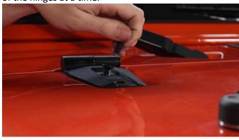
With the respective bracket and two of the included bolts and spacers, place the bracket into place as shown. Once level, secure it to the vehicle with a 5mm Allen wrench.
