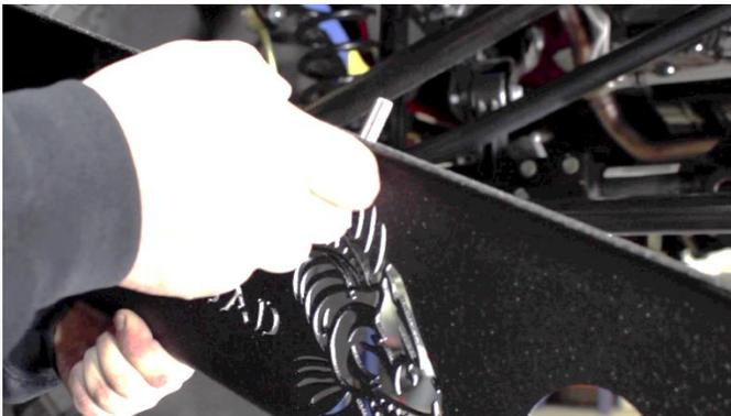
With your factory skid plate mounting bolts, secure the two plate brackets to the frame with a 16mm
