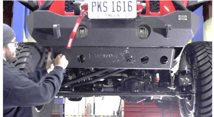
Install the included hardware into the remaining 5 skid plate and Mako bumper holes. With a 5mm allen key and a 13mm wrench, secure the skid plate to the bumper.
