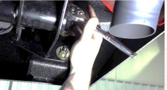
Secure the center of the bumper to the frame with the remaining (2) counter sunk bolts with an 8mm Allen key.
