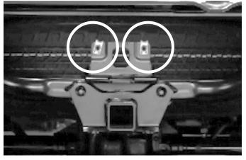
3) INSTALL YOUR MAKO BUMPER Slide the Mako into the frame mounting holes.
