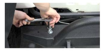
Remove only the two (2) front stabilizer mounting bolts. DO NOT remove the stabilizer mounting bolts that are located between the stabilizer bar and the grille.
