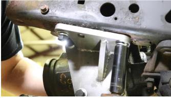
NOTE: When reinstalling the hanger bracket, ensure the bracket sits in between the mount and the frame, and the remaining spacer is used with the rear most bolt to level out the plate.
