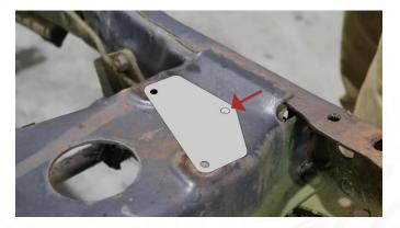
With a 1/2" drill bit, drill out the marking.
