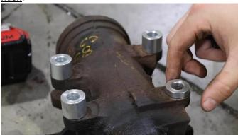
Thick spacers will require a shoulder bolt and washers, while the thin spacer will require a large hex bolt and washers. Secure them with a 5/8" socket.
