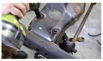
Remove the mount from the box by removing the remaining two hex bolts with a 5/8'' socket, followed by the two inverted torx bolts with an E14 inverted torx bit.
