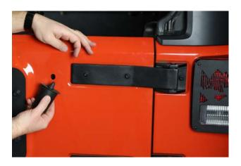
Insert the two smaller grommets into the rubber stopper holes.
