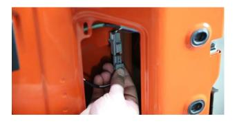
Pull the third brake light wire harness through the tailgate by pushing the grommet out from the inside of the tailgate while gently pulling the harness from the outside.
