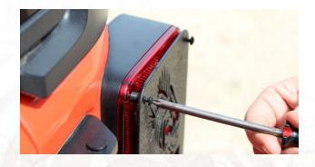
Tighten screws with the screwdriver. **DO NOT OVERTIGHTEN!**
