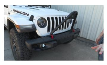
Once centered, finish tightening the bolts with a T40 torx bit.
