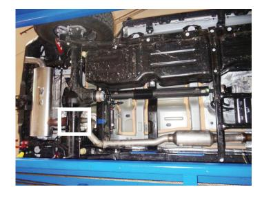
5. Remove muffler from vehicle.
