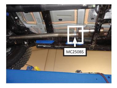
13. Place clamp (MC250BS) onto inlet of over-axle pipe (86506S). Connect over-axle and front pipes while pushing wire hanger into rubber isolator on vehicle. Tighten clamp just enough to allow for adjustment.
