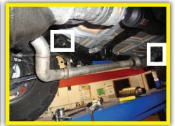
8. Remove resonator assembly from vehicle and retain clamp for re-use.
