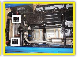
4. Secure and support muffler, then loosen clamp at muffler inlet connection above rear axle.
