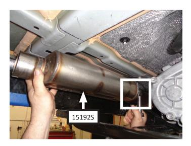
12. Place **clamp (MC250BS)** onto outlet of resonator. Connect front pipe to resonator. Make sure the bend on front pipe is oriented upwards as shown. Tighten clamp just enough to allow for adjustment.
