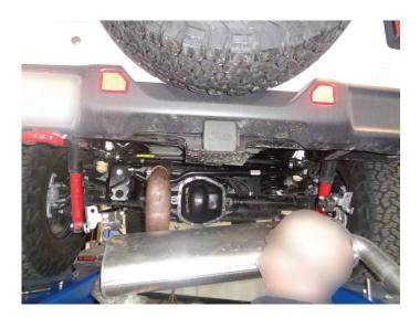
6. Place stock muffler next to Outlaw **muffler** (842583-511) oriented in the same direction. Then transfer driver and passenger side mounts over.
