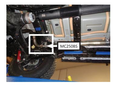
14. Place **clamp (MC250BS)** onto inlet of muffler. Connect muffler to over-axle pipe. Support muffler and ensure all connections are completely seated.
