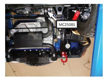
15. Place muffler hanger mounts into position, then reinstall and tighten factory bolts. (removed steps 2 and 3).
