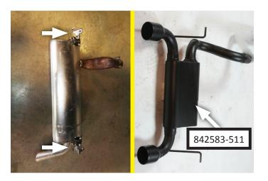
7. Remove wire hanger on resonator assembly from isolator, and loosen bolt on clamp at resonator inlet.
