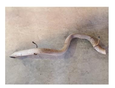
6. Remove nuts (x2) from flanges then remove factory muffler from vehicle.
