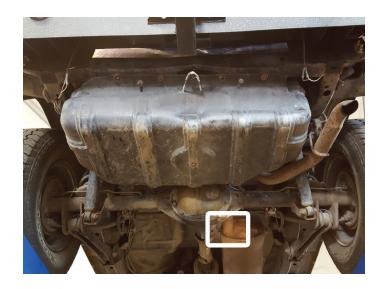
5. Dismount factory tailpipe wire hangers then remove tailpipe from vehicle.
