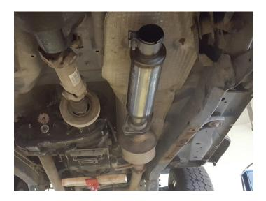
9. Route **tailpipe (86563M)** over axle and connect it to muffler outlet. Mount wire hangers into isolators (x2) then tighten clamp enough to allow for adjustment.
