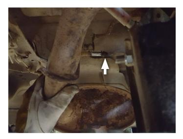
4. Cut tailpipe just behind factory muffler then remove completely from vehicle.
