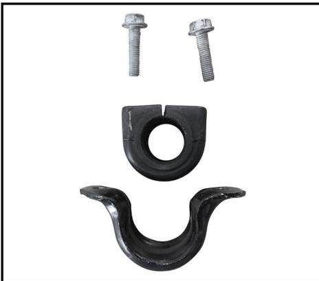
**FIGURE 3: OEM Bushing and Mounting Install**
