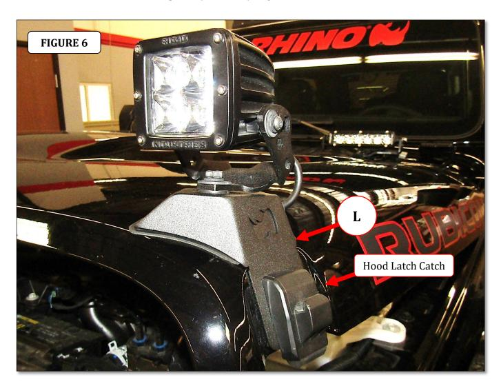
**Step-16** Repeat the above steps to install the LED light and bracket assembly on the passenger side of the vehicle.
