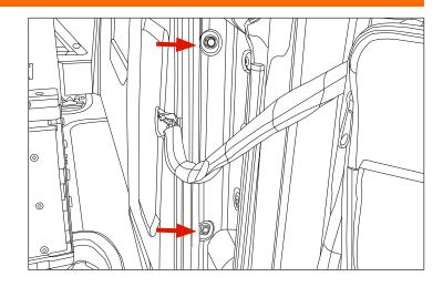
7. The tailgate strut is located on the bottom of the tailgate. Using a small flat head screw driver, lift retainer clip on tailgate strut. Gently pull strut away from ball bracket on tailgate.
