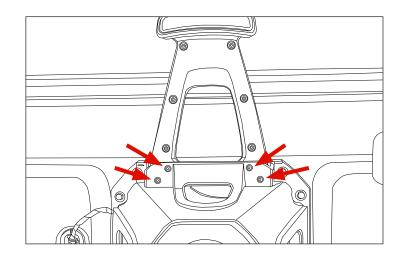
22. Align the OE tire carrier to the tailgate. Using only the passenger side mounting holes (1), loosely attach the tire carrier reusing OE hardware.
