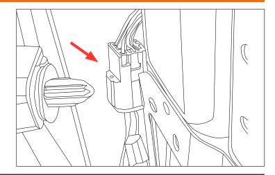
10. Pull the plug toward you. Press down on the plug release and pull to diconnect it from the vehicle.
