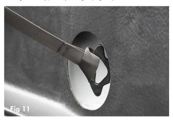
**4-**Wrap the long strap piece around an opposite side truck bed corner cleat, thread its end through its loop, and pull tight.
